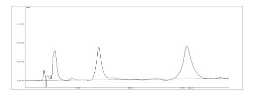
Fig. 2: Representative Chromatogram of standard solution of Glycyrrhetinic acid at  $15.4 \pm 0.2$  min and Forskolin  $7.0 \pm 0.2$  min.
