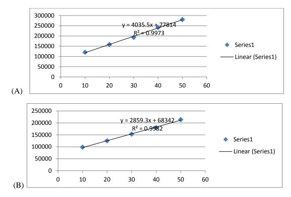
Fig. 3: calibration curve for linearity of Glycyrrhetinic acid(A) and Forskolin(B) 10-50 (µg/ml)
